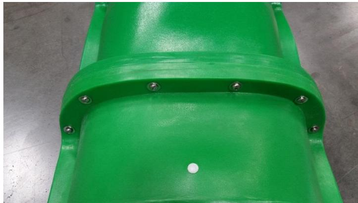
3. Repeat Step 2 across all of the inserts. When you are ready to join the bottom piece, you will need to raise the slide in order to properly align the two sections.
